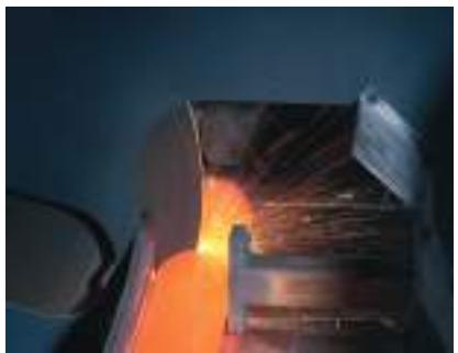
**Market leader in the steel industry** — We are the most sought-after producer of the world's biggest cut-off wheels with diameters of up to 2,000 mm for cutting hot semi-finished steel products.
